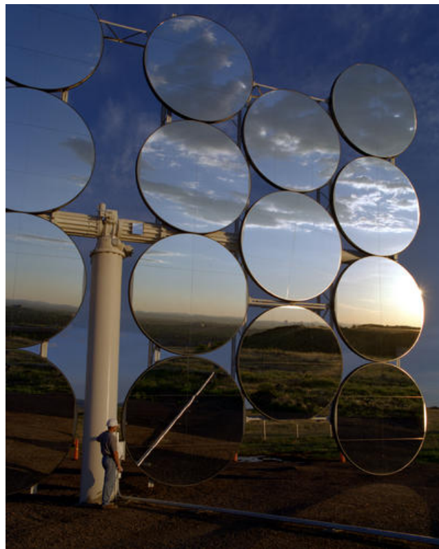
24 25 FIGURE 5.12-10 Heliostats for a Solar Power 26 Tower (Credit: W. Getz; Source: NREL 2009b)
